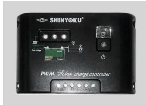
Figure 4 The Shinyoku solar charge controller
