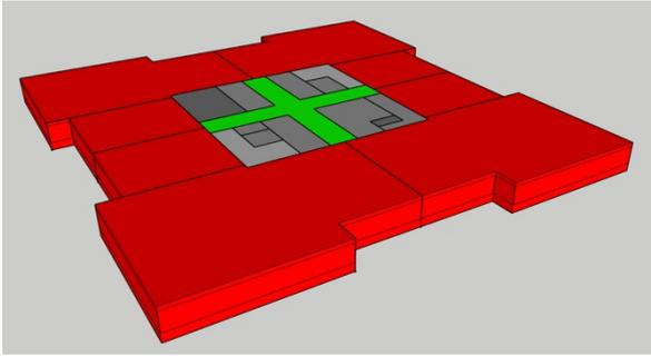
Figure 2. Base Design Model, Conditioned Zone: Open Office in Red and Internal Corridor in Green
