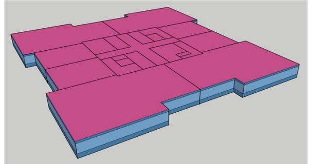
Figure 3. Base Design Model: Ceiling and Floor Set as Adiabatic
